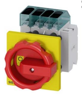
Switch disconnector 3LD3, main switch 3-polig + N, lu 25A operational switch at AC-23 A at 400 V 9,0 kW front mounted Base mounting with center-hole 22,5 mm knob-operated mechanism red/yellow 66 x66 mm with auxiliary 1NO+1NC
