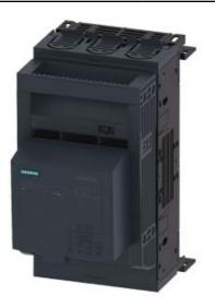
FUSE-SWITCH-DISCONNECTOR 3-POLE, NH00, 160A 60MM BUSBAR SYSTEM COVER LEVEL 32/70 MM FLAT CONNECTOR FUSE MONITORING ELECTRONIC, EFM 10
