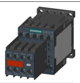
CONTACTOR, AC-3, 5.5KW/400V, 2NO+2NC, DC 24V, W. INTEGRATED DIODE 3-POLE, SZ S00 SCREW TERMINAL PERMANENT AUX. SWITCH
