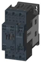
CONTACTOR, AC-3, 7.5KW/400V, 1NO+1NC, AC 24V 50/60HZ, 3-POLE, SZ S0 SPRING-LOADED TERMINAL
