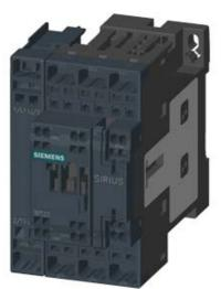
4NO CONTACTOR, AC1: 40A DC 125V 4-POLE, 4NO, SZ: S0, SPRING-LOADED TERMINAL 1NO+1NC INTEGR.
