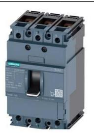
CIRCUIT BREAKER 3VA1 IEC FRAME 100 BREAKING CAPACITY CLASS B ICU=16KA @ 415 V 3-POLE, LINE PROTECTION TM210, FTFM, IN=80A OVERLOAD PROTECTION IR=80A FIXED SHORT CIRCUIT PROTECTION II=10 X IN BUSBAR CONNECTION
