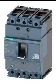
CIRCUIT BREAKER 3VA1 IEC FRAME 160 BREAKING CAPACITY CLASS S ICU=36KA @ 415 V 3-POLE, LINE PROTECTION TM220, ATFM, IN=20A OVERLOAD PROTECTION IR=14A ...20A SHORT CIRCUIT PROTECTION II=16 X IN BUSBAR CONNECTION
