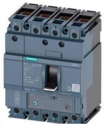
CIRCUIT BREAKER 3VA1 IEC FRAME 160 BREAKING CAPACITY CLASS N ICU=25KA @ 415 V 4-POLE, LINE PROTECTION TM240, ATAM, IN=25A OVERLOAD PROTECTION IR=17,5A ...25A SHORT CIRCUIT PROTECTION II=5...10 X IN NEUTRAL UNPROTECTED CABLE CONNECTION
