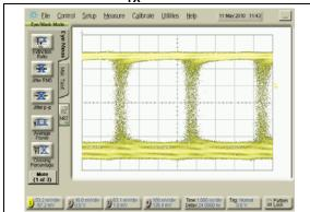
FIGURE B-4: 1.485 Gbps, 200m,  $\Delta V_{TX}$  = 620 mV
