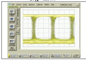
FIGURE B-2: 270 Mbps, 410m,  $\Delta V_{TX} = 800 \text{ mV}$
