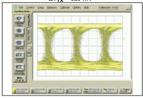
FIGURE B-5: 1.485 Gbps, 200m,  $\Delta V_{TX} = 800 \text{ mV}$
