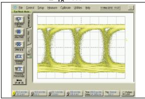
FIGURE B-6: 1.485 Gbps, 200m,  $\Delta V_{TX} = 980 \text{ mV}$
