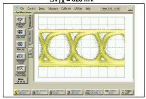
FIGURE B-8: 2.97 Gbps, 140m,  $\Delta V_{TX} = 800 \; mV$
