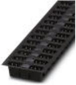
Header, Nominal current: 12 A, Rated voltage (III/2): 320 V, Number of positions: 4, Pitch: 5 mm, Color: black, Contact surface: Tin, Mounting: THR soldering, The maximum current depends on the plug used. The lower of the two current values apply for plug and pin strip. The pin strip is made of highly temperature resistant plastic and is thus suitable for the reflow process.
