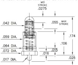
0930 - Spring-Loaded Pin Packaging: Packaged in Bulk **Durability:**
