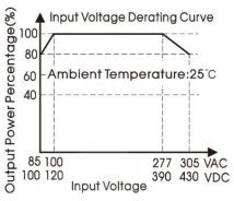
Note: ① With an AC input between 85-100V/277-305VAC and a DC input between 100-120VDC/390-430VDC, the output power must be derated as per
