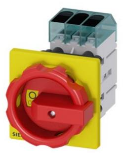
Switch disconnector 3LD3, main switch 3-polig, Iu 25A operational switch at AC-23 A at 400 V 9,0 kW front mounted Base mounting with center-hole 22,5 mm knob-operated mechanism red/yellow 66 x66 mm
