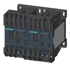
REV. COMB., AC3, 5.5KW/ 400V AC230V, 50/60 HZ, 3-POLE, SZ S00 SPRING-LOADED TERMINAL ELECTR. AND MECH. INTERLOCK
