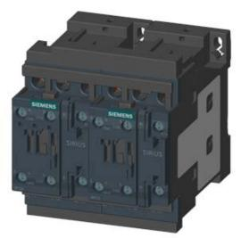
REV. COMB. FOR 3RA27, AC3, 5.5KW/400V, DC24V 3-POLE, SZ S0 SCREW TERMINAL ELECTR. AND MECH. INTERLOCK 2NO INTEGR.
