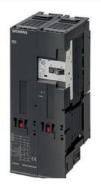
RS1-X FOR ET 200S ELECTRO-MECH. REVERS. STARTER, EXPANDABLE SETTING RANGE 2.2...3.2A AC-3, 1.1KW/400V
