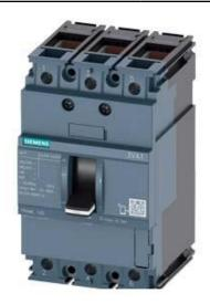
CIRCUIT BREAKER 3VA1 IEC FRAME 100 BREAKING CAPACITY CLASS N ICU=25KA @ 415 V 3-POLE, LINE PROTECTION TM210, FTFM, IN=80A OVERLOAD PROTECTION IR=80A FIXED SHORT CIRCUIT PROTECTION II=10 X IN CABLE CONNECTION
