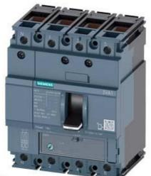
CIRCUIT BREAKER 3VA1 IEC FRAME 160 BREAKING CAPACITY CLASS H ICU=70KA @ 415 V 4-POLE, LINE PROTECTION TM220, ATFM, IN=32A OVERLOAD PROTECTION IR=22,4A ...32A SHORT CIRCUIT PROTECTION II=10 X IN NEUTRAL PROTECTION 100% CABLE CONNECTION
