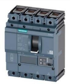
CIRCUIT BREAKER 3VA2 IEC FRAME 160 BREAKING CAPACITY CLASS C ICU=110KA @ 415 V 4POLE, LINE PROTECTION ETU850, LSI, IN=160A OVERLOAD PROTECTION IR=64A ...160A SHORT CIRCUIT PROTECTION ISD=0,6..10X IN, II=1,5..10X IN NEUTRAL PROTECTION ADJUSTABLE (OFF, UPTO 100%) CABLE CONNECTION
