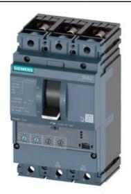
CIRCUIT BREAKER 3VA2 IEC FRAME 250 BREAKING CAPACITY CLASS L ICU=150KA @ 415 V 3POLE, LINE PROTECTION ETU330, LIG, IN=160A OVERLOAD PROTECTION IR=64A ...160A SHORT CIRCUIT PROTECTION II=1,5...12 X IN GROUNDFAULTPROTECTION IG=0,2... 1 X IN, TG=0,1/0,3MS BUSBAR CONNECTION
