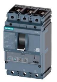
CIRCUIT BREAKER 3VA2 IEC FRAME 250 BREAKING CAPACITY CLASS C ICU=110KA @ 415 V 3POLE, LINE PROTECTION ETU330, LIG, IN=250A OVERLOAD PROTECTION IR=100A ...250A SHORT CIRCUIT PROTECTION II=1,5...10 X IN GROUNDFAULTPROTECTION IG=0,2... 1 X IN, TG=0,1/0,3MS BUSBAR CONNECTION
