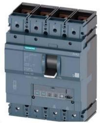
CIRCUIT BREAKER 3VA2 IEC FRAME 630 BREAKING CAPACITY CLASS H ICU=85KA @ 415 V 4-POLE, LINE PROTECTION ETU350, LSI, IN=400A OVERLOAD PROTECTION IR=160A ...400A SHORT CIRCUIT PROTECTION ISD=1,5... 10 X IR, II=12 X IN NEUTRAL PROTECTION ADJUSTABLE(OFF,50%,100%) BUSBAR CONNECTION
