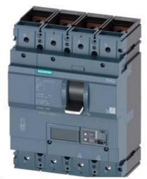
CIRCUIT BREAKER 3VA2 IEC FRAME 630 BREAKING CAPACITY CLASS M ICU=55KA @ 415 V 4-POLE, LINE PROTECTION ETU850, LSI, IN=500A OVERLOAD PROTECTION IR=200A ...500A SHORT CIRCUIT PROTECTION ISD=0,6..10X IN, II=1,5..14X IN NEUTRAL PROTECTION ADJUSTABLE (OFF, UPTO 100%) BUSBAR CONNECTION
