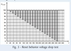
Verify the behavior of a DUT during and after cranking.
