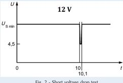
Fig. 2 - Short voltage drop test
