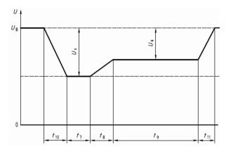
Fig. 1 - Motor startup curve
