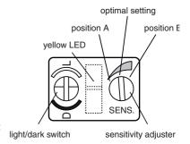
· For optimal setting, now turn the sensitivity adjuster to the middle position between the positions A and B.
