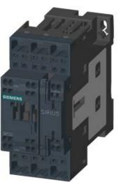
CONTACTOR, AC-3, 15KW/400V, 1NO+1NC, DC 24V, 3-POLE, SZ S0 SPRING-LOADED TERMINAL
