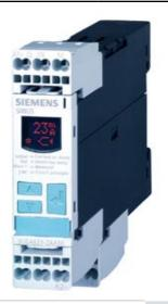
OVERSHOOT AND UNDERSHOOT SUPPLY VOLTAGE: AC/DC 24V DC AND AC 50 TO 60 HZ NO GALVANIC ISOLATION FROM MEASURING CIRCUIT STARTUP AND INTERF. PEAK DELAY 0.1 TO 20S HYSTERESIS 0.1 TO 250MA 1 CO CONTACT W. OR W/O ERROR LOG AUTOM. RESET SPRING-LOADED CONNECTION
