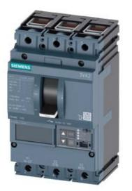
CIRCUIT BREAKER 3VA2 IEC FRAME 100 BREAKING CAPACITY CLASS M ICU=55KA @ 415 V 3POLE, LINE PROTECTION ETU560, LSIG, IN=25A OVERLOAD PROTECTION IR=10A ...25A SHORT CIRCUIT PROTECTION ISD=0,6..10X IN, II=1,5..12X IN NEUTRAL PROTECTION OPTIONAL WITH EXT. CT,UPTO 160% GROUNDFAULT, SWITCHABLE IG=0,2... 1 X IN, TG=0,050,8MS CABLE CONNECTION
