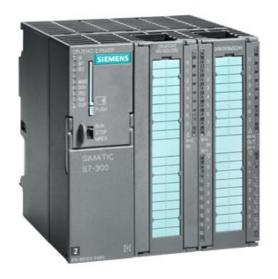
SIMATIC S7-300, CPU 314C-2PN/DP COMPACT CPU WITH 192 KBYTE WORKING MEMORY, 24 DI/16 DO, 4AI, 2AO, 1 PT100, 4 FAST COUNTERS (60 KHZ), 1. INTERFACE MPI/DP 12MBIT/S, 2. INTERFACE ETHERNET PROFINET, WITH 2 PORT SWITCH, INTEGRATED 24V DC POWER SUPPLY, FRONT CONNECTOR (2 X 40PIN) AND MICRO MEMORY CARD REQUIRED
