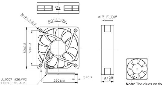
Note: The glues on the impeller is for impeller balance. Do not remove it.
