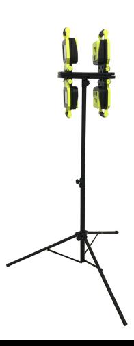
The TRIPOD-360 is a solid tripod that can hold up to 4 Unilite site lights at once, with 2 being placed on the top and 2 underneath. It can be dropped to 960 mm or raised to 1930 mm via the ergonomic grips.
