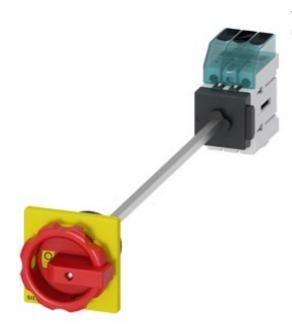
Load disconnector 3LD3, Iu 32 A Main switch 3-pole Rated operating capacity for AC-23 A at 400V 11.5kW floor mounting Basic switch with door coupling Central hole mounting 22.5mm Rotary actuator red / yellow 66 x 66 mm
