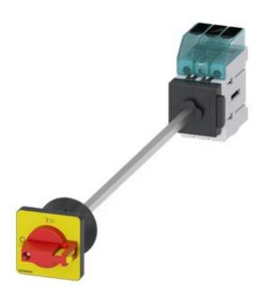
Switch disconnector 3LD3, main switch 3-polig, Iu 25A operational switch at AC-23 A at 400 V 9,0 kW floor mounting Base mounting with door coupling center-hole 22,5 mm knob-operated mechanism red/yellow  $48 \times 48 \text{ mm}$
