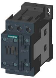
CONTACTOR, AC-3, 18.5KW/400V, 1NO+1NC, AC(50-60HZ)/DC ACTUAT. AC/DC 95...130V, 3-POLE, SZ S0 SCREW TERMINAL
