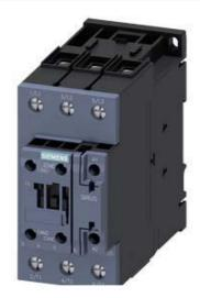
CONTACTOR,AC3:30KW/400V, 1NO+1NC, 208V AC 50/60HZ, 3-POLE, SIZE S2, SCREW TERMINAL
