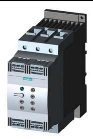
SIRIUS SOFT STARTER, S3, 80A, 45KW/400V, 40 DEGR., AC 200-480V, AC/DC 24V, SPRING-LOADED TERMINALS, THERMISTOR MOTOR PROTECTION
