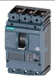
CIRCUIT BREAKER 3VA2 IEC FRAME 100 BREAKING CAPACITY CLASS L ICU=150KA @ 415 V 3POLE, LINE PROTECTION ETU550, LSI, IN=25A OVERLOAD PROTECTION IR=10A ...25A SHORT CIRCUIT PROTECTION ISD=0,6..10X IN, II=1,5..12X IN NEUTRAL PROTECTION OPTIONAL WITH EXT. CT,UPTO 160% BUSBAR CONNECTION
