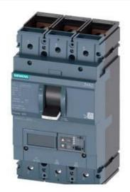
CIRCUIT BREAKER 3VA2 IEC FRAME 400 BREAKING CAPACITY CLASS C ICU=110KA @ 415 V 3-POLE, LINE PROTECTION ETU560, LSIG, IN=400A OVERLOAD PROTECTION IR=160A ...400A SHORT CIRCUIT PROTECTION ISD=0,6..10X IN, II=1,5..10X IN NEUTRAL PROTECTION OPTIONAL WITH EXT. CT;UPTO 160% GROUND-FAULT, SWITCHABLE IG=0,2... 1 X IN, TG=0,05-0,8MS BUSBAR CONNECTION
