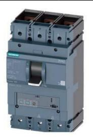
CIRCUIT BREAKER 3VA2 IEC FRAME 630 BREAKING CAPACITY CLASS C ICU=110KA @ 415 V 3-POLE, LINE PROTECTION ETU320, LI, IN=400A OVERLOAD PROTECTION IR=160A ...400A SHORT CIRCUIT PROTECTION II=12 X IN BUSBAR CONNECTION
