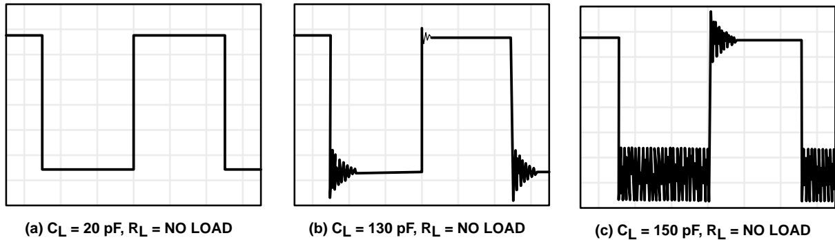
Figure 110. Effect of Capacitive Loads in High-Bias Mode
