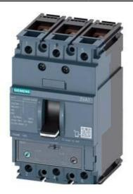
CIRCUIT BREAKER 3VA1 IEC FRAME 160 BREAKING CAPACITY CLASS N ICU=25KA @ 415 V 3-POLE, LINE PROTECTION TM240, ATAM, IN=100A OVERLOAD PROTECTION IR=70A ...100A SHORT CIRCUIT PROTECTION II=5...10 X IN BUSBAR CONNECTION
