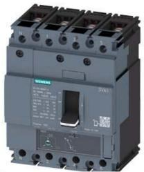
CIRCUIT BREAKER 3VA1 IEC FRAME 160 BREAKING CAPACITY CLASS N ICU=25KA @ 415 V 4-POLE, LINE PROTECTION TM220, ATFM, IN=100A OVERLOAD PROTECTION IR=70A ...100A SHORT CIRCUIT PROTECTION II=10 X IN NEUTRAL PROTECTION 100% BUSBAR CONNECTION
