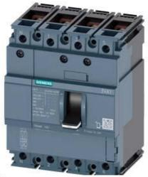
CIRCUIT BREAKER 3VA1 IEC FRAME 160 BREAKING CAPACITY CLASS N ICU=25KA @ 415 V 4-POLE, LINE PROTECTION TM210, FTFM, IN=160A OVERLOAD PROTECTION IR=160A FIXED SHORT CIRCUIT PROTECTION II=10 X IN NEUTRAL UNPROTECTED BUSBAR CONNECTION
