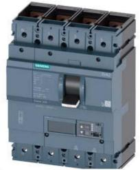
CIRCUIT BREAKER 3VA2 IEC FRAME 630 BREAKING CAPACITY CLASS M ICU=55KA @ 415 V 4-POLE, LINE PROTECTION ETU850, LSI, IN=400A OVERLOAD PROTECTION IR=160A ...400A SHORT CIRCUIT PROTECTION ISD=0,6..10X IN, II=1,5..15X IN NEUTRAL PROTECTION ADJUSTABLE (OFF, UPTO 160%) BUSBAR CONNECTION
