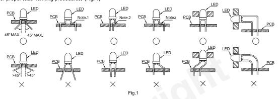
"O" Correct mounting method "imes" Incorrect mounting method
