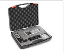
Powerful digital force gauge with graphic assisted display for tensile and compressive force measurements with external load cell
