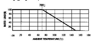
**Technical data:** Rated power: 0.5 W (Derating from Ta=70°C) • Tolerance: 1% • Temp.-range: -30 ... 150 °C • Working voltage: 350 V • Dielectric withstanding/overload voltage: max. 700 V • Temp. Coefficient max  $\pm 100$  ppm/°C • Solder ability: Dip the lead in to a solder bath having a Temperature of 260 °C  $\pm 5$  °C up to 4  $\pm 0.8$ mm from the body of the resistor and hold it for 5  $\pm 0.5$  seconds then inspect.
