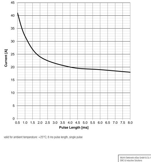
**Typical Peak Current vs. Pulse Length Characteristics:**
