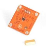
**Output**: This module outputs 5v when the slider is at one end and 0v when moved in the opposite way. When connected to an input on the Arduino using the TinkerKit Shield, you can expect to read values going from 0 to 1023.
