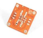
This module is a **SENSOR**. The connector is an **OUTPUT** which must be connected to one of the **INPUT** connectors on the **TinkerKit Shield**.
