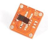
**Module description**: On the back of the module you can find two signal amplifier and a green LED that signals that the module is correctly powered. The module is based on the <u>LIS344AL</u> by ST Microelectronics, and is a three-axis acceremoter. You can get data about the third axis (referred to as Z) by soldering a header to the thru-hole labeled "Z".
