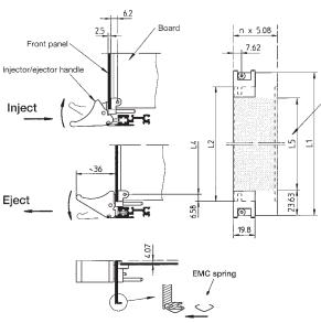
Injector/Ejector Handle With Locking Feature (Function)
